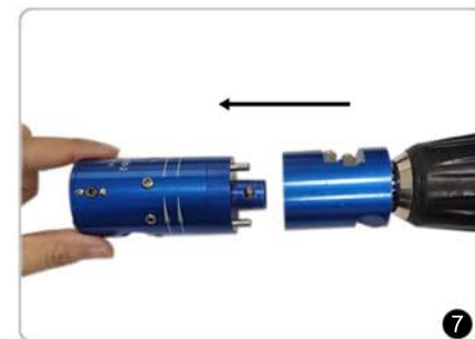
Remove the front part of trimming tool from the base. The base will remain attached to the drill.
