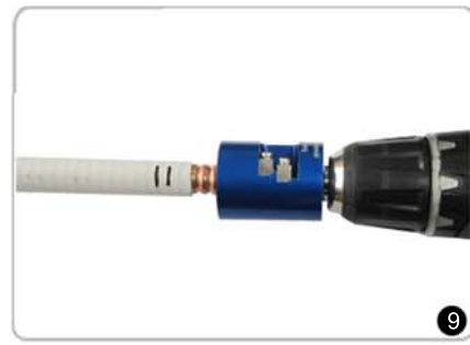
To prevent damage to the cable, do not push the trimming tool beyond the end of the cable jacket.
