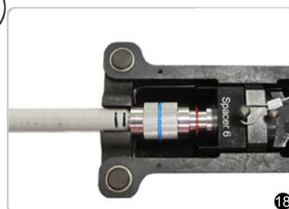
18 Make sure the connector nut is lined up against spacer 6 to prevent damage to the O-ring during compression.
