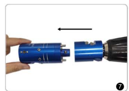
Disassemble the front part from trimming tool. The back part of trimming tool remains assemble to the power drill.
