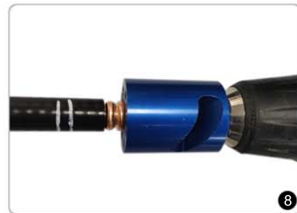
Using the low speed setting on the drill, insert exposed outer conductor into trimming tool base. Continue trimming until tool reachscable jacket. Do not push tool beyond this point.
