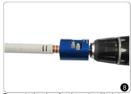
To create the chamfer shown in critical step, push the power drill with back part of trimming tool at low speed or 400 RPM until the leading surface of trimming tool reaches the cable jacket.
